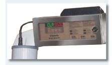
GREEN AND RED METERING SIGNALS PROPORTIONAL TO THE METAL MASS DETECTED
