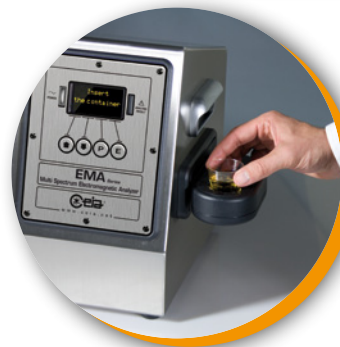
INSERTION OF THE SAMPLE CUP INTO THE EXTERNAL PROBE
