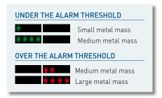
✓ Green and Red Metering Signals Proportional to the Metal Mass Detected Enhanced Multi-Zone Metal Detector
