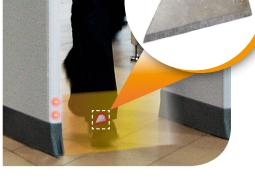
Light bars indicate metal position vertically and laterally and can also show pacing lights
